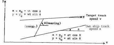
One Bearing Given At time  $t_1$ , bearing  $\beta_1$  is observed. Thus,
